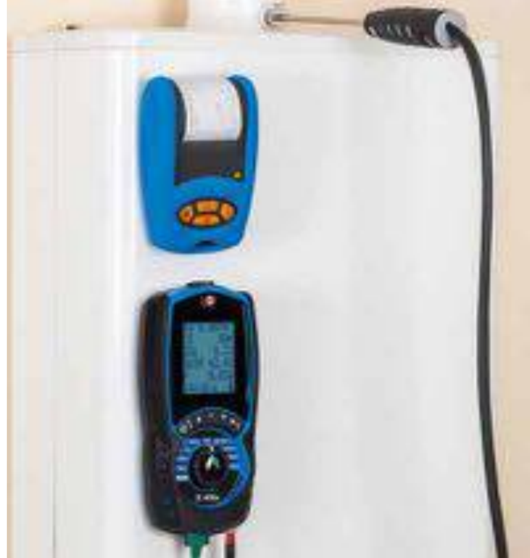
Flue Gas Analysis
